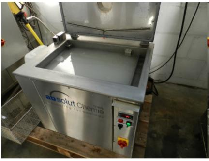
Old coating needs to be removed prior to deposition of coating particularly to gear cutting tools.
