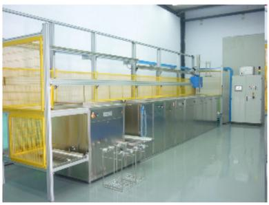
Water cleaning with nine tanks and drying module meets modern international standards. Elements of cleaning plant are as follows:
